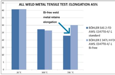
Comparison between Bi-containing and Bi-free 347 type weld metal. At high temperatures, the Bi-free weld metal retains its elongation properties.
